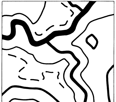
6. Scale 1:500,000, contour interval 200 meters, good generalization. Enlarged to 1:50,000.
