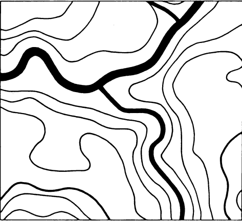
3. Scale of 1:200,000, contour interval 100 meters, poor generalization. Enlarged to 1:50,000.
