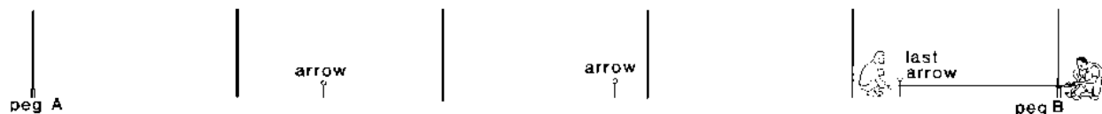
Fig. 16c Measurement of a long distance, Step 4
